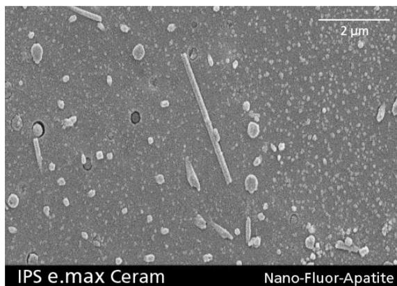
Fig. 1: Microstructure of IPS e.max Ceram (SEM image): fluorapatite crystals in different sizes
