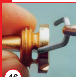
46 Push the new retaining ring...
