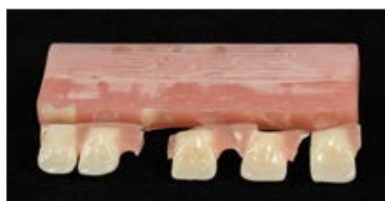
Figure 15 a: Fracture pattern; tooth base was sandblasted and coated with bonding agent
