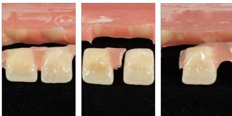
Figure 14 a – c: Typical fracture pattern after bond testing of VITA PHYSIODENS with the base materials named above (Base material from left to right: FuturaGen, ProBase Cold, PalaXpress)
