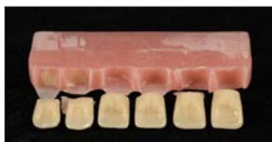
Figure 15 c: Fracture pattern; tooth base was only conditioned by sandblasting
